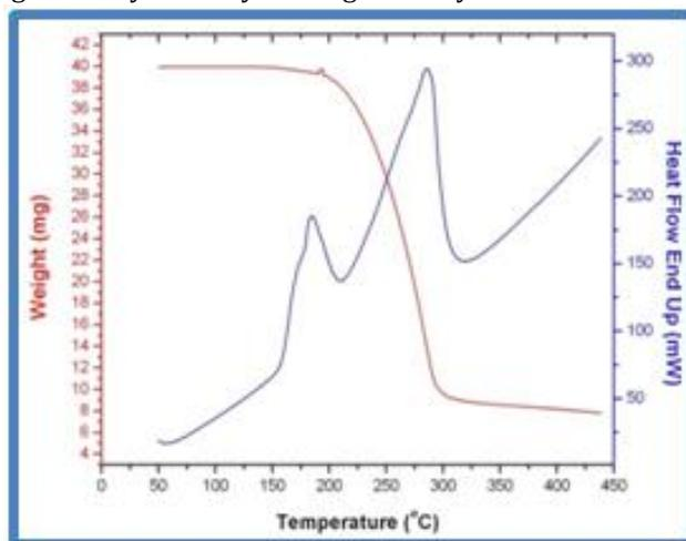
Figure 11 TGA and DSC curves of grown OS crystals
