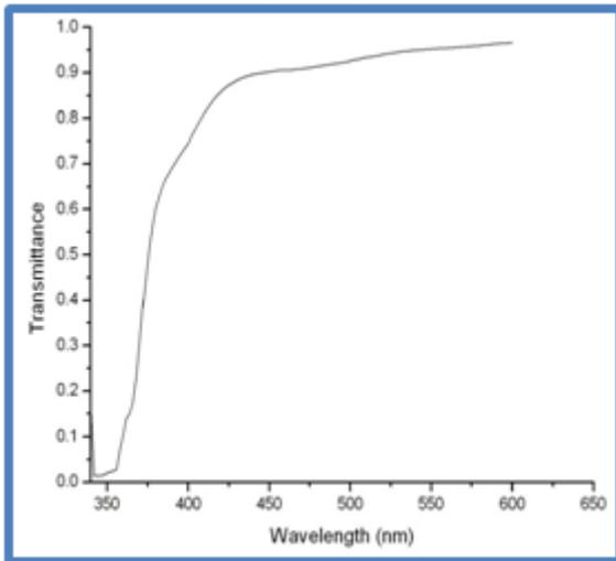
Figure 6 UV-visible transmission spectrum of grown OS crystal.
