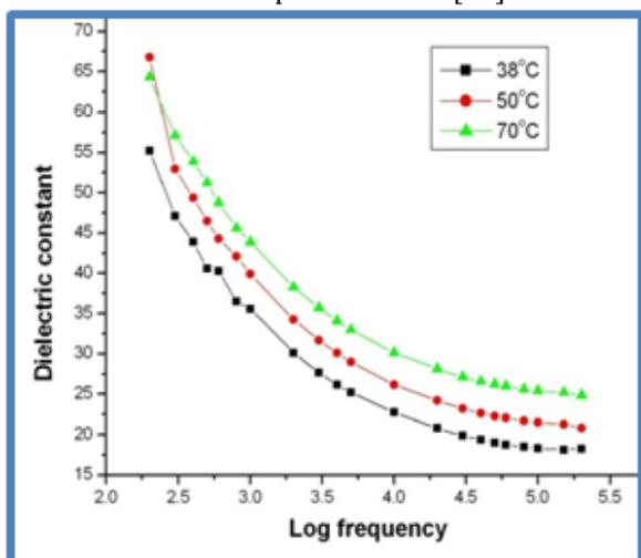
Figure 9 The plot of dielectric constant ( $\epsilon_r$ ) vs. log frequency of OS crystal
