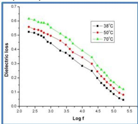
Figure 10 The plot of dielectric loss vs. log frequency of OS crystal.
