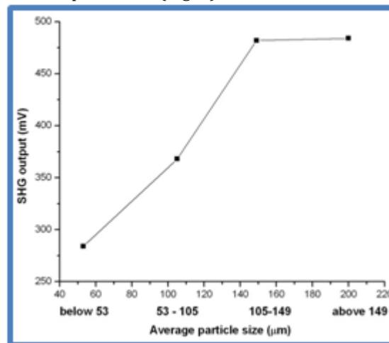
**Figure 8** The plot of the SHG output values vs. average particle size of OS crystal.
