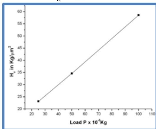
**Figure 12** Variation of Vicker microhardness with applied load of OS crystal.
