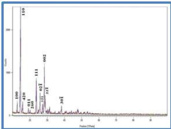
**Figure 3** X-ray powder diffraction pattern of the OS crystals.
