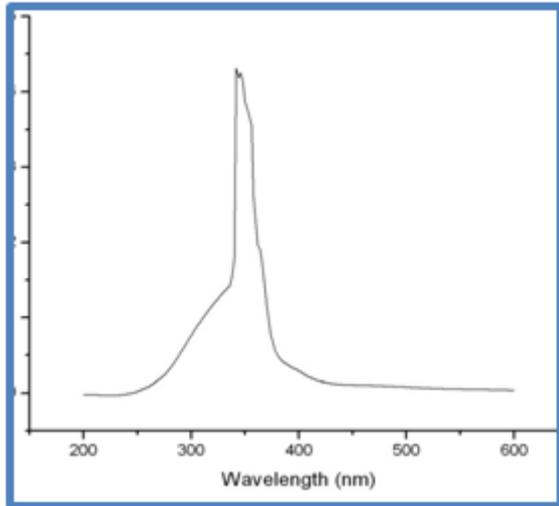
Figure 5 UV-visible absorption spectrum of the OS crystal.
